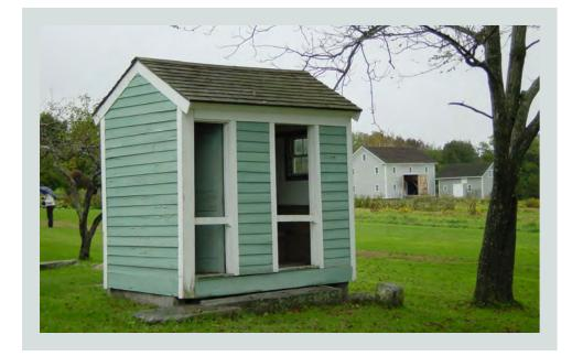
Located within the stone foundation wall, which is all that remains of the 1794 Ministry Barn, is this small clapboarded privy measuring 6.5 x 13 feet. The clapboarded privy consists of two equal-sized compartments, accessed by single doors on the south side of the building.
